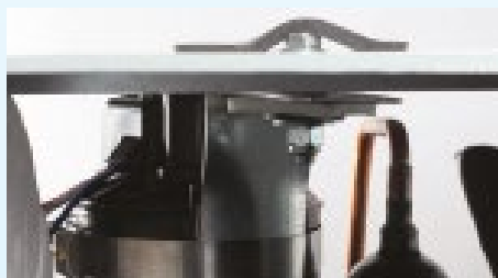
Compressor is bracketed at top and bottom to minimise vibration and movement
