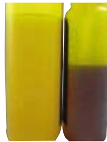
TRACER® additives (right) contain 10 times more dye than other UV additives(left)
